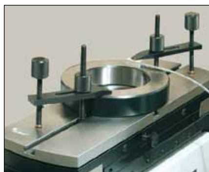
Temperature compensation system TempComp
