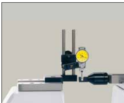
Checking of test indicators (TULM15)
