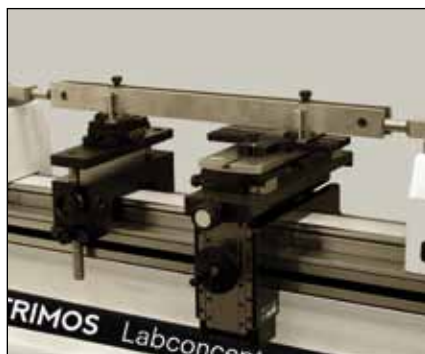
Comparative checking of gauge blocks > 250 mm (TA-SU-313/TELMA7/P/TA-SU-305/TA-SU-306)
