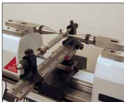
Calibration of thread plug gauges (HPA-1/TEL6/3P/0.17-3.2/S6.5/LABC-15)
