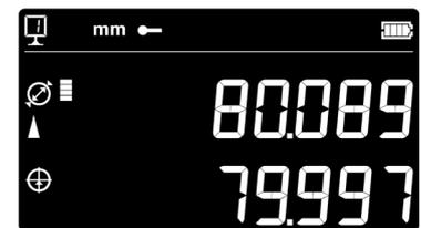
4b. Probe a point near the reversal point on the side opposite the diameter (4). Move the part (or the instrument) laterally to determine the reversal point (5). Remove the measuring insert to the side, off centre (6). Diameter and centreline values are displayed on the 1<sup>st</sup> and 2<sup>nd</sup> lines of the display respectively.
