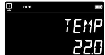
Enter the value of thermal expansion coefficient of the part (value between 0 and 200, unit [ $10^{-6} \text{ K}^{-1}$ ]) and confirm by pressing *Validation Key*.
