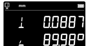
For a new perpendicularity measurement, restart from point 5. To quit this mode, press again *validation key*.
