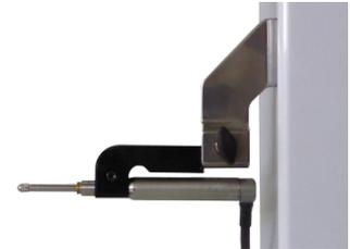
3. Place the part to be measured against the probe, taking care that the contact is maintained on the whole part to be measured. Bring the carrier to its starting position.
