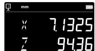
5. Initialize display by pressing the zero setting key. The measurement starts as the key is pressed.
