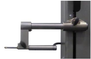
2. Connect the perpendicularity probe to the measuring column.
