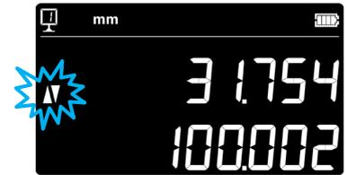
2. Set the display at zero or at a preset value with the measuring insert probing a reference surface (see § 5.11 and § 5.4.2).
