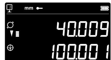
5. When the measuring insert is removed, the display remains frozen on the diameter and centerline values.
