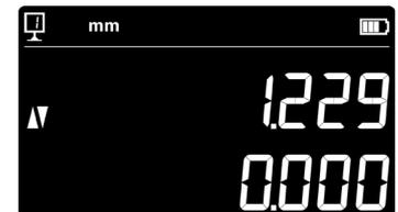
If the same key is pressed for more than 2 seconds, the current position of the probe will be initialized to the preset value of the current reference, regardless of the last probing.
