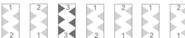
In case of odd number of teeth use indexable insert No 3 once
