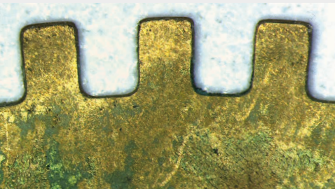
Oxidation on gear wheel
