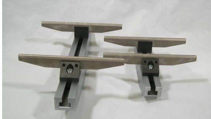
4-point bend jig with extended-width fins
