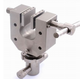
Mec154-20-Ni – nickel plated Temperature range -70 to +350°C
