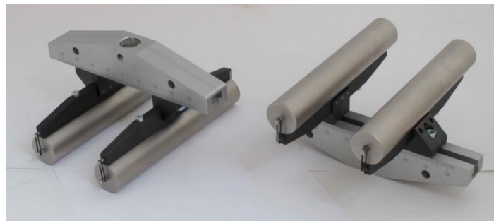
4-point bend jig with large diameter wide anvils
