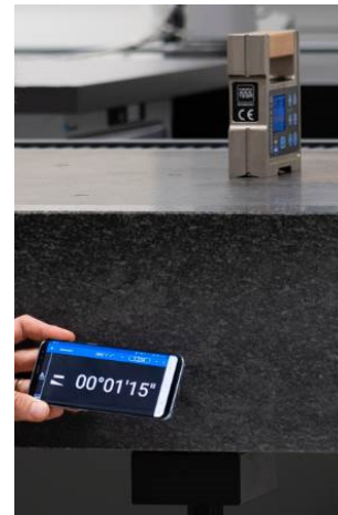
TESA CLINOBEVEL 3 with an Android device as remote display
