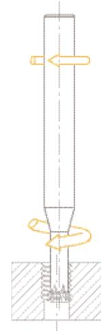
MACHINING ON A SWISS-TURNING MACHINE - Workpiece turns
