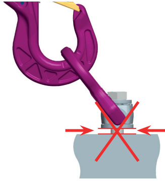
Fig. 5: The lifting point must have been fully bolted in.
