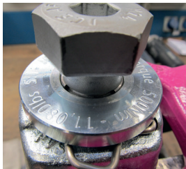
Fig. 12: Circlip fully positioned in the recess of the countersink
