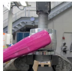
Fig. 10: Supporting position of the ACP on of the vice jaws
