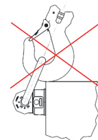
Pic. 5: Forbidden contact or support at/or with edge
