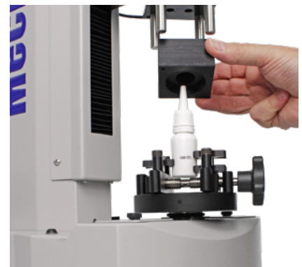
PSV18155 V-Jaw with Toggle Clamp (Tornado/Orbis/Vortex)
