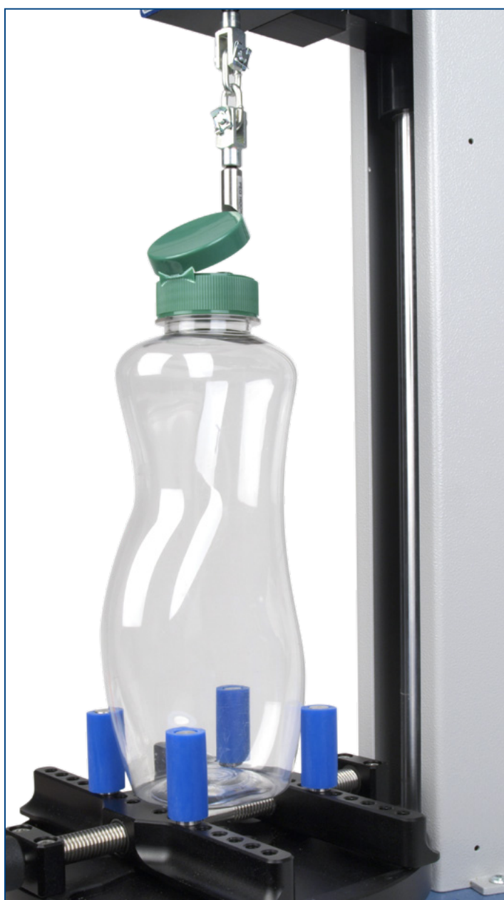
▲ 432-411 Large 4-peg container holder, plastic bottle application
