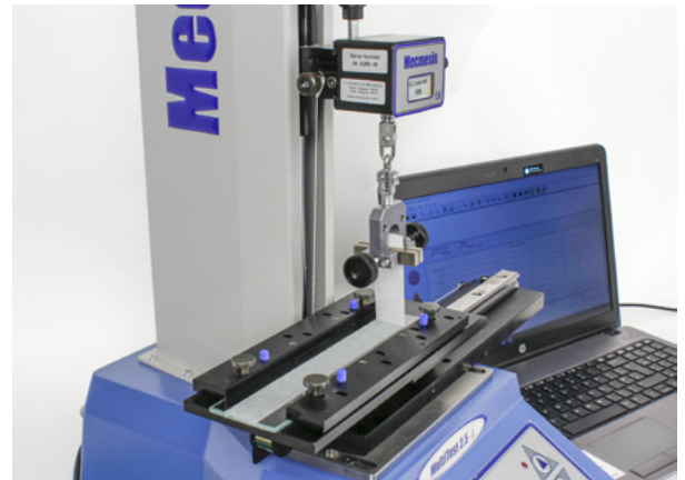
▲ Pull-Peel Table (PDV15031) shown with 25mm strip being held in Upper Grip (Mec227-BG50)
