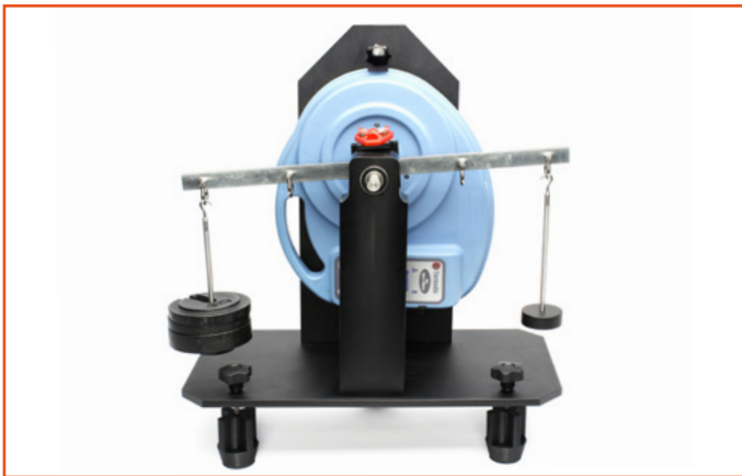
Checks gauge torque cells
