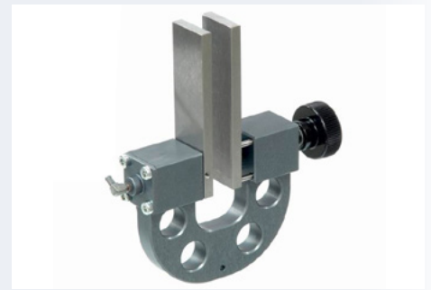
Mec94 with Mec94-B100x25 special blank jaws
