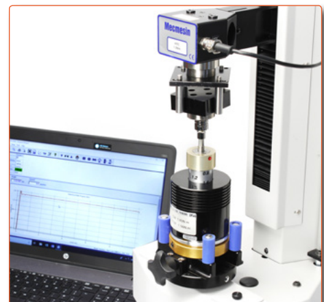
Torque value check on Helixa
