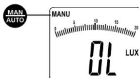
measuring range. Press the „MAN/AUTO“ button until the corresponding manual measuring range is set or until „AUTO“ appears in the display, indicating that the automatic measuring range is set again.
